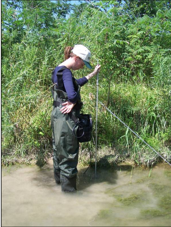
Fig 2.13: Streamgauging with a) the Flo-Mate apparatus; and b) the bridge apparatus at Boyd Creek Hwy. 21 overpass.
