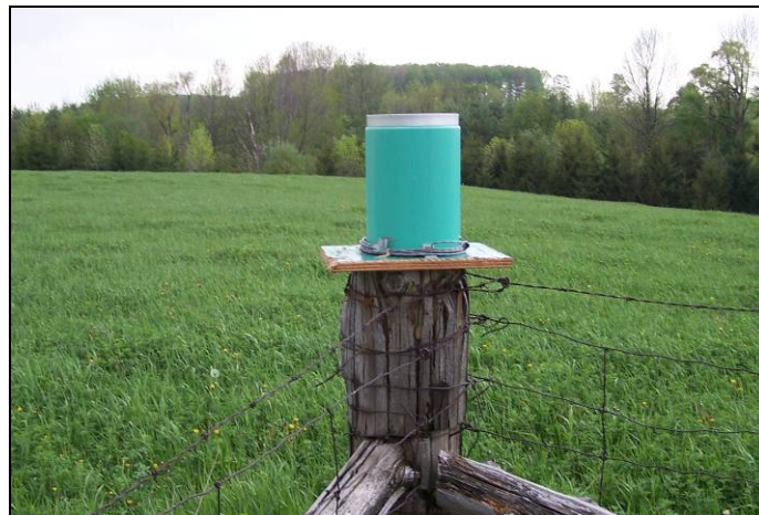
Fig 1.4: Manual Rain Gauge at Ashfield-Colborne-Wawanosh Service Garage
